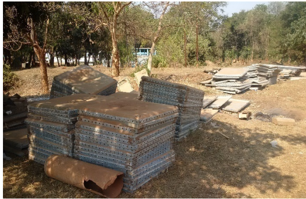
Panels Replaced from Ngwenya tank at LWB Yard
