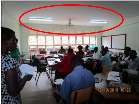
Figure 11: Insufficient natural lighting at HTC Mulago
